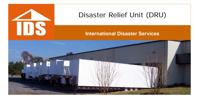
The Disaster Relief Unit, or DRU for short, is a temporary housing and utility unit designed for immediate deployment after disasters. It can be delivered quickly and installed virtually anywhere. The unit is constructed from 40' trans-modal cargo containers, giving it strength, durability, and ease of transport.
